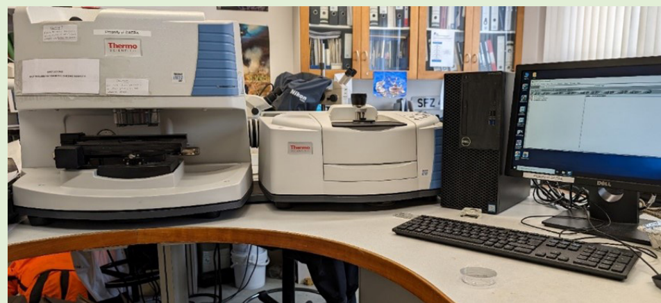
Image of FTIR machine used in our microbead analysis.
