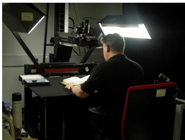
Overhead mounted digital camera system used at PRONI for digitising archival material
