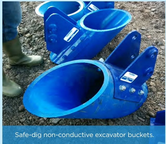
The plastic bucket avoids potential excavating headaches and safety issues.
