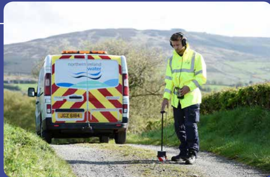
Leakage detection in Omagh, County Tyrone
