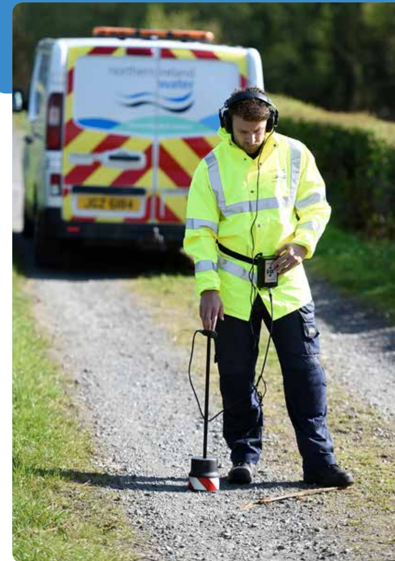
Leakage detection in Omagh, County Tyrone
