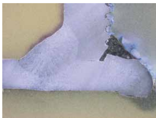
Picture of a defective weld under magnification
