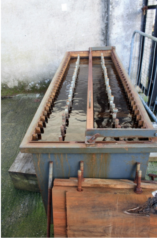
Tank for soaking paddles. The tank was designed and made by Waterways Ireland
