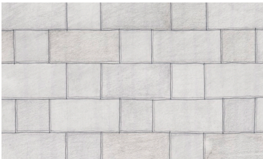
Block in course Used in walls built for strength. Stones are deeper than usual. Stones shorter on the face are long stones running back into the depth of the wall
