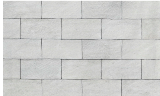
Ashlar Regular squared fine-jointed work which looks similar to Block-in-course but stones are not as deep
