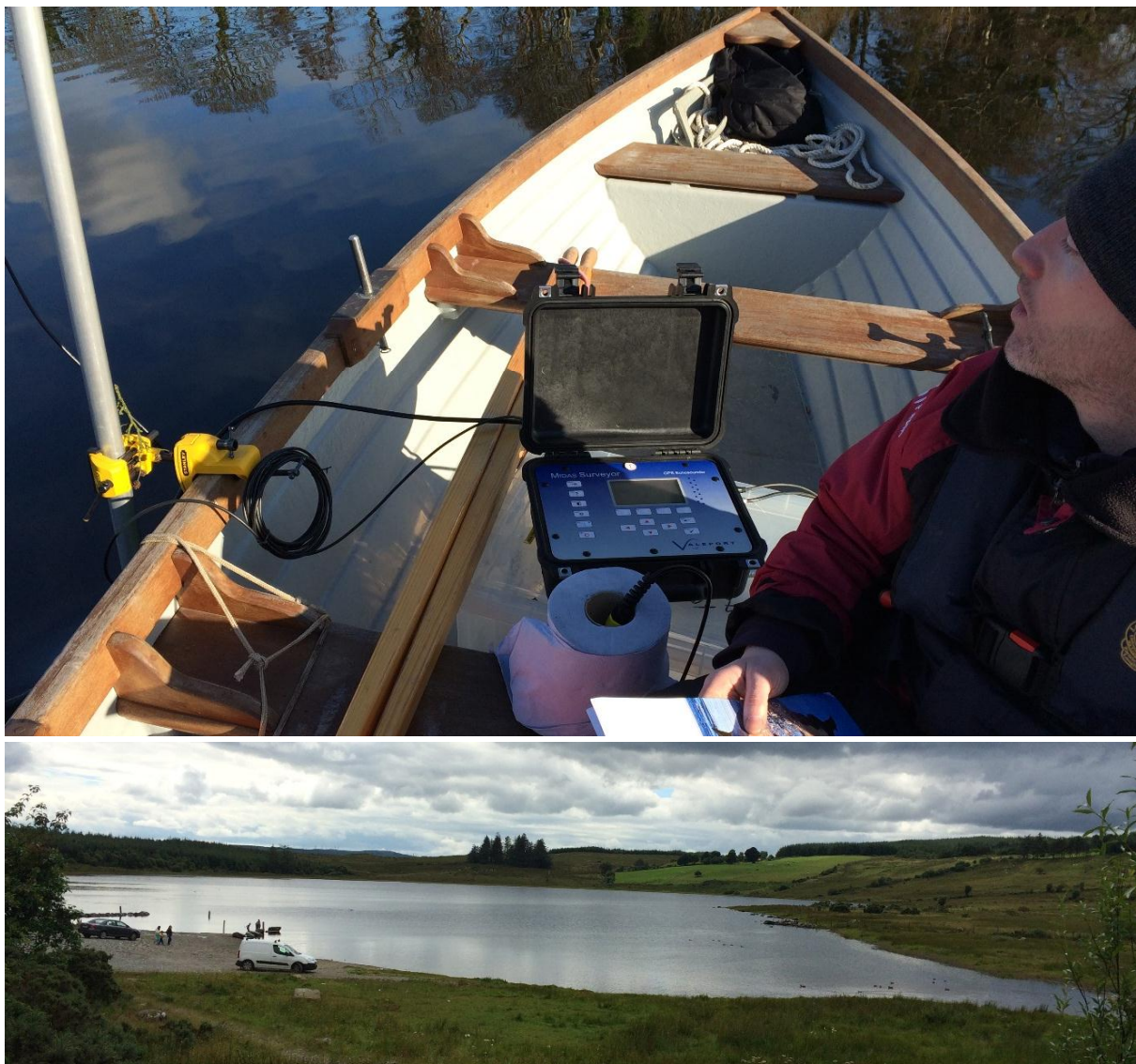
Fig 2. Echo sounder recording data points during the bathymetry survey of the lough
