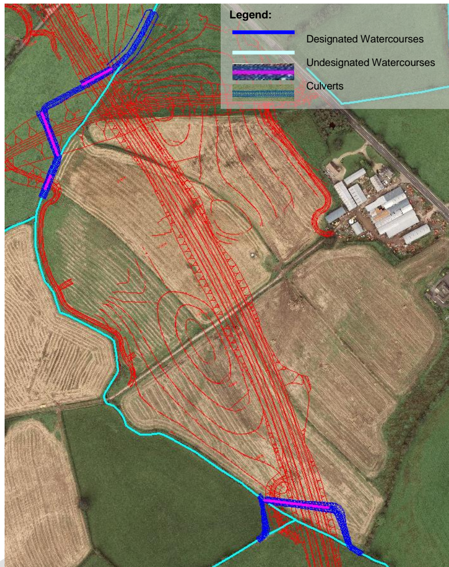
Figure 4.15.2-1 - Plan of Ranelly Drain Diversion (S3-WD-04, S3-WD-05 and S3-WD-46) and Culvert Arrangement (S3-PC-06, S3-PC-74, S3-PC-82 and S3-PC-53)
