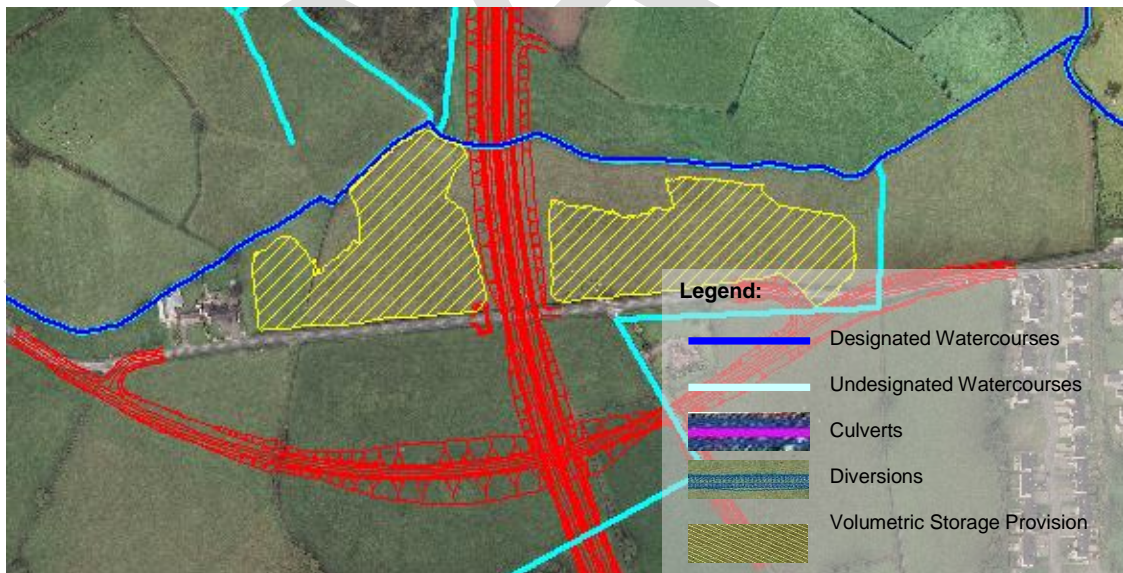
Figure 4.12.3-3 – Model M.4, Plan of Omagh Volumetric Floodplain Storage Provision (S2-CS-11 and S2-CS-12)
