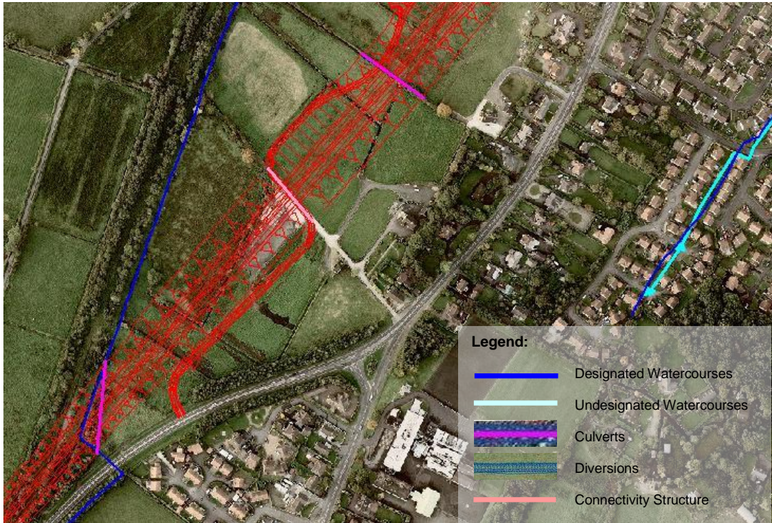
Figure 4.5.2-7 - Plan of Backfence Drain and Field Drain Culvert Arrangement; Culvert (S1-PC-18 and S1-PC-19) and Connectivity Culvert (S1-CC-05)
