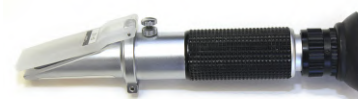
Figure 28: A useful on farm tool for measuring the concentration of immunoglobulins in colostrum is a Brix refractometer and so can aid in the overall picture of colostrum management in the herd.
