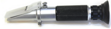
Figure 106: A useful on farm tool for measuring the concentration of immunoglobulins in colostrum is a Brix refractometer and so can aid in the overall picture of colostrum management in the herd.
