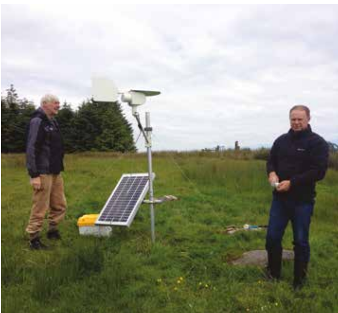
Burkard spore sampler: sampling for aerial spread of fungal spores
