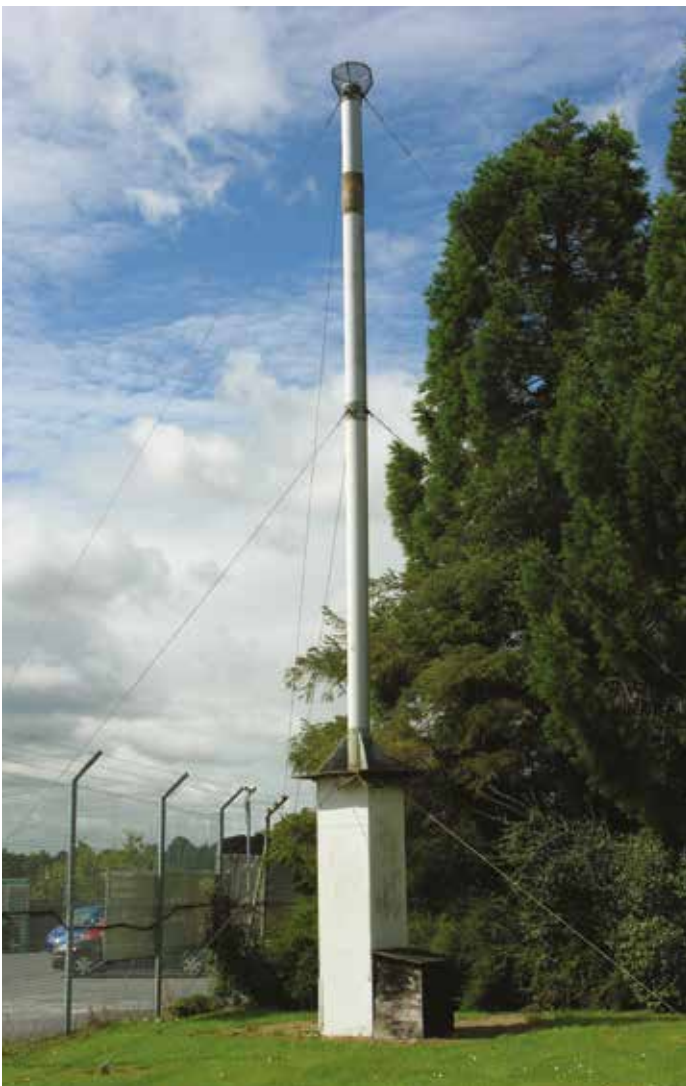
Belfast suction trap: aerial sampling for insects
