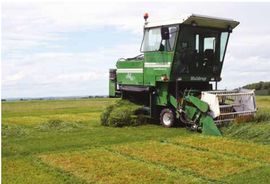
New grass plot harvester with on-board NIRS scanner for herbage quality
