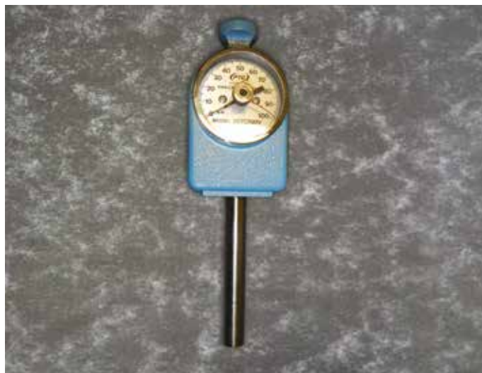
A durometer has been successfully used to test for shell softness in brown crab.
