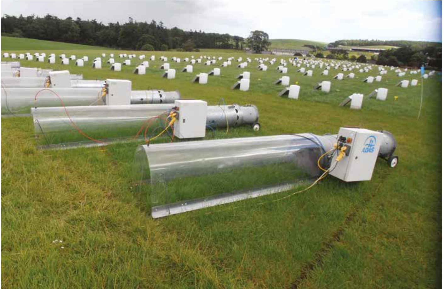
Measuring gaseous emissions at AFBI Hillsborough as part of the UK GHG Inventory Programme.
