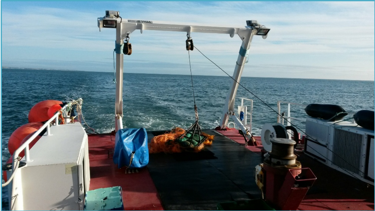
Figure 2: Photograph showing the mussel dredge used during the Spring 2017 survey.
