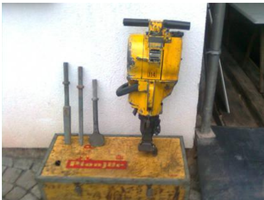
Pionjar deep overburden sampling device
