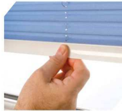
Tensioned pleated blind - all cords are held under tension and the blind is just pushed or pulled into position
