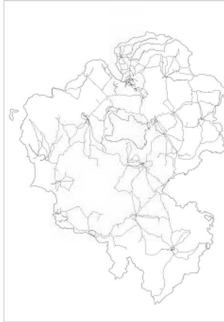
33kV Distribution Network in NI
