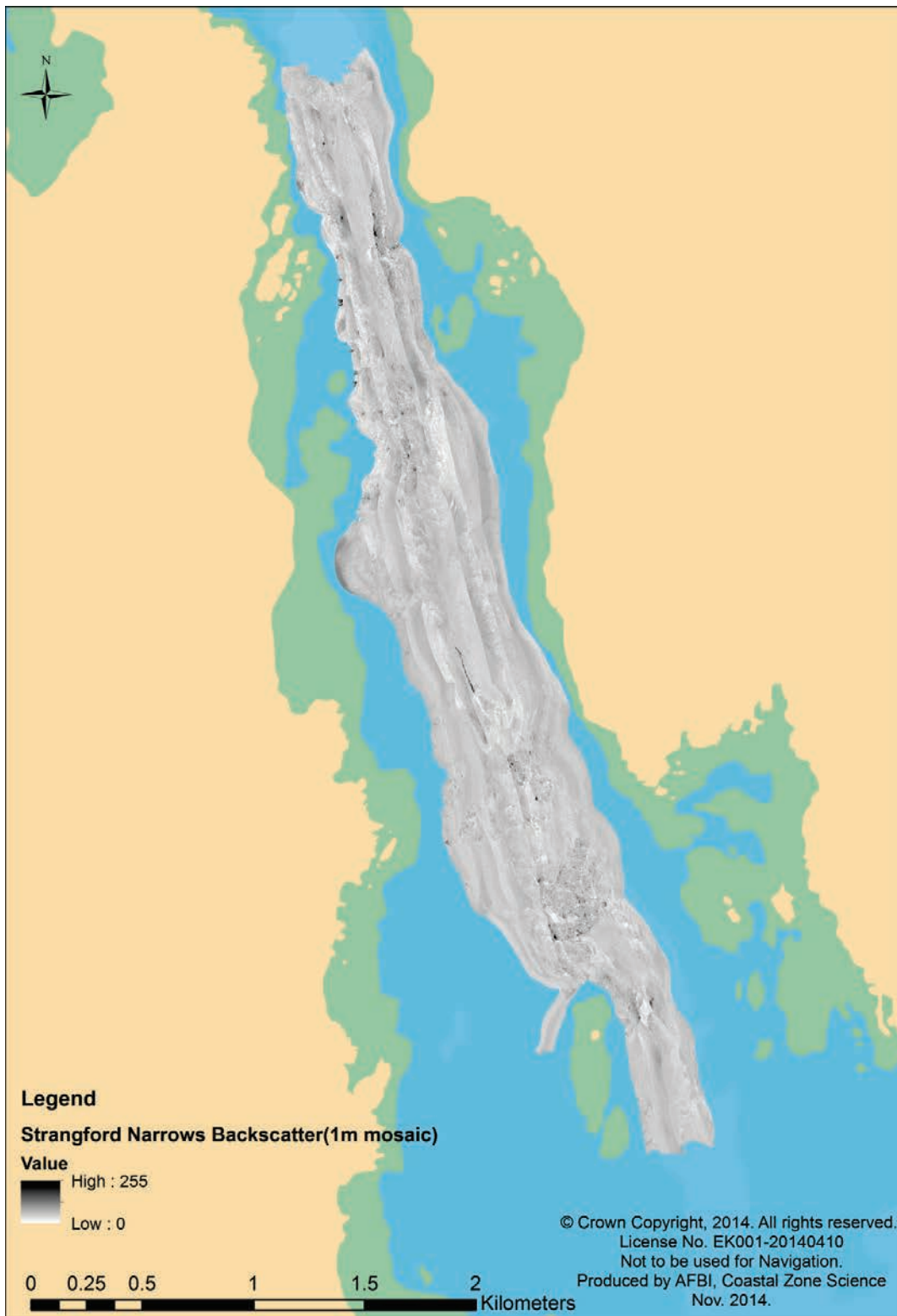
Figure 3.4 Multibeam backscatter mosaic for the Narrows. Low image values = high reflectivity (coarser or harder ground), high image values = lower reflectivity (softer ground).
