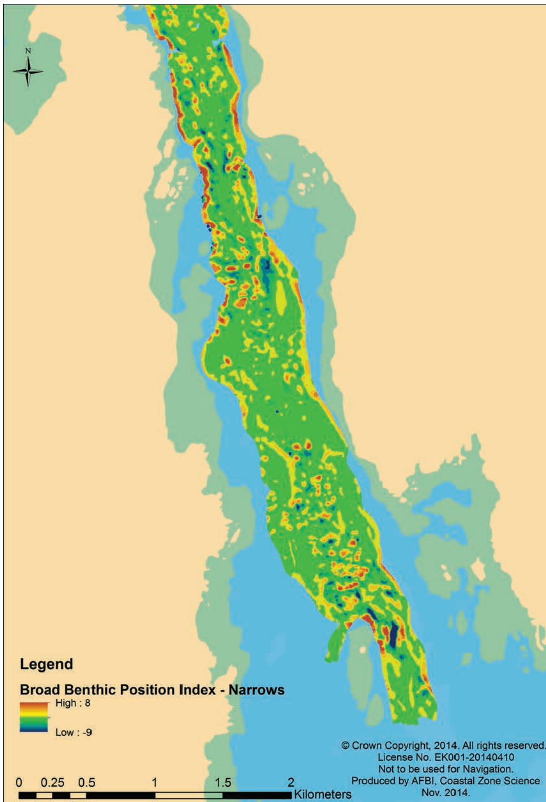
Figure 3.10. Broadscale benthic position index (BPI) for the Narrows with crest areas shown as high positive values and trough areas shown as high negative values.
