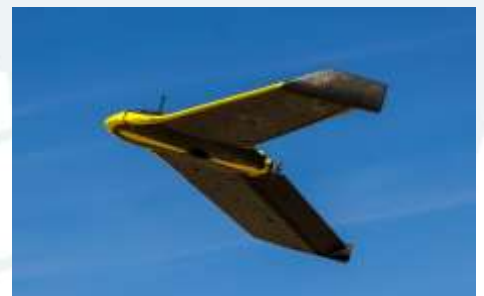
Figure 2. Sensfly eBee UAV
