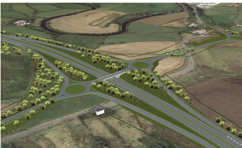
Indicative Grade-Separated Junction
