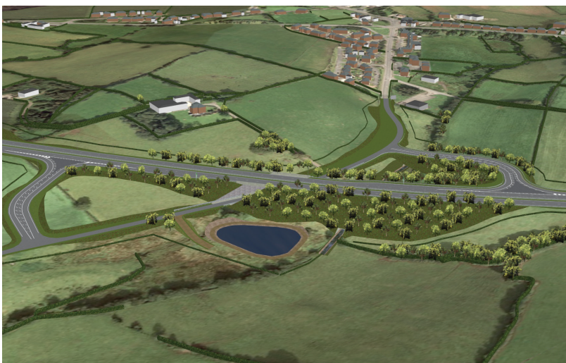
Indicative Compact Grade-Separated Junction
