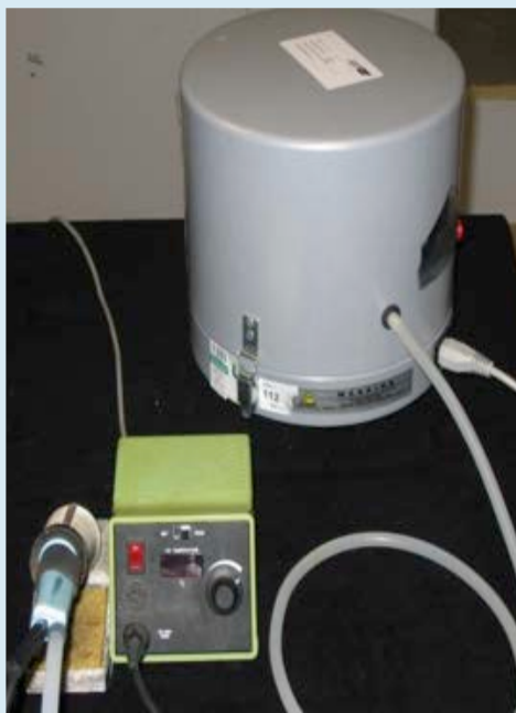
Figure 4 An on-tip solder fume extraction system
