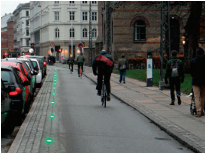
Figure 18 (Bottom left): Modular LED running lights help cyclists maintain proper travel speed so that they maintain effort required for green wave and they don't have to stop at the red light.
