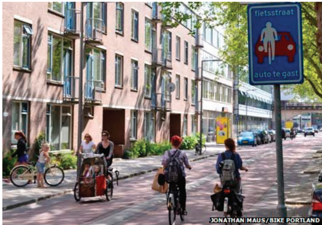
Figure 3: A typical Fietsstraat in the Netherlands, This shows both the signage used and colouring of the road surface.
