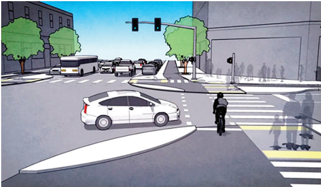
Figure 5: A common Dutch signalised Junction
