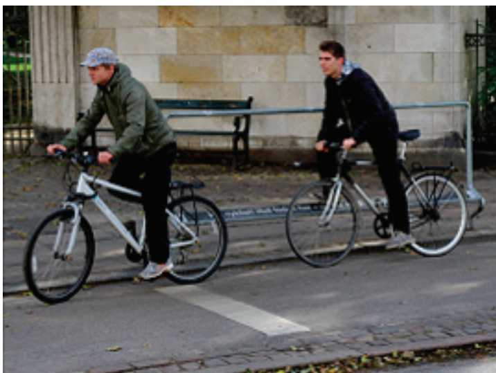
Figure 19 (Below): Foot rests at signalised intersections provide added comfort when cyclists do have to stop.
