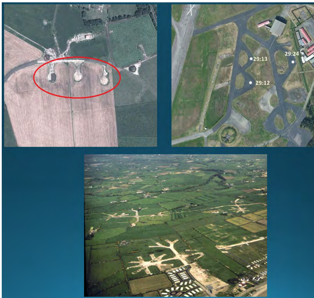
Figure 5. Frying Pan dispersals at Limavady, Co. Londonderry (DHR 00070), Spectacle dispersals at Ballykelly, Co. Londonderry (DHR 00029) and Finger Park dispersals at Greencastle, Co. Down (DHR 00039)
