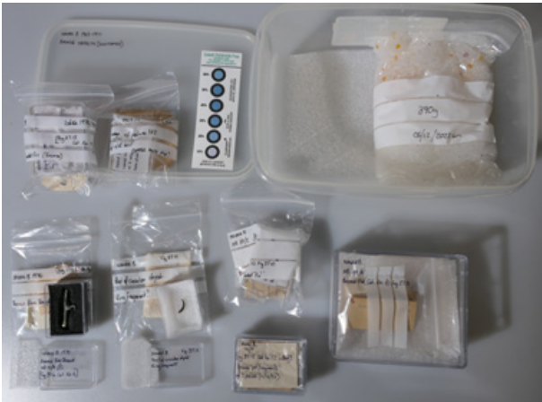
Individual metal artefacts, packed and ready to be placed into a larger box with silica gel and a humidity indicator card
