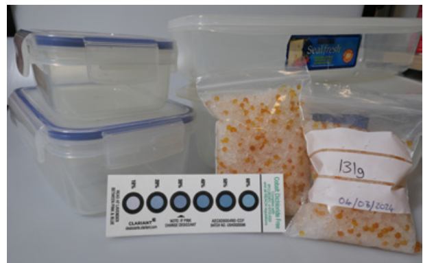
Examples of packaging materials for metal objects, including airtight boxes, silica gel (both indicating and non-indicating mix in perforated and labelled bags) and a humidity indicator card
