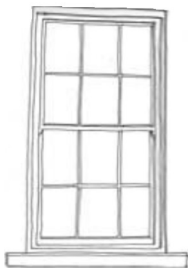
Six-over-six Sash window
