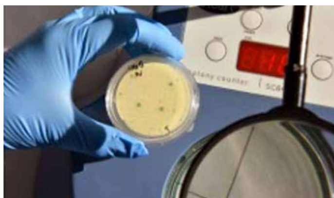
Figure 3 Counting faecal bacterial growth on agar plates.
