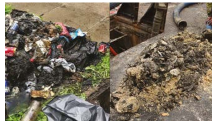
Figure 7 - Rubbish items and a fatberg recovered from sewers
