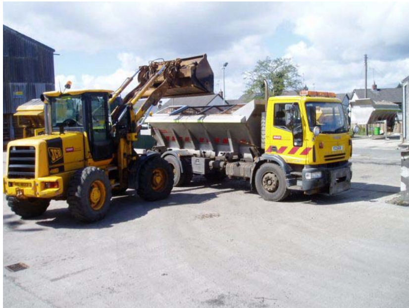
Loading a lorry for a gritting action
