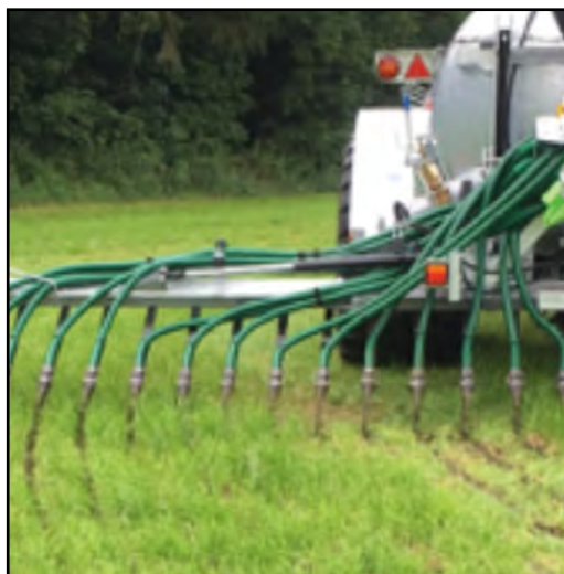
Photo 3 - Trailing shoe spreader
