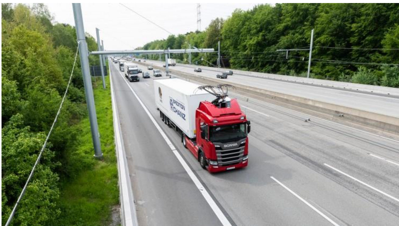
Figure 2-6 - Battery ERS HGV driving on an Electric Road System 'eHighway' (source: Siemens [11])
