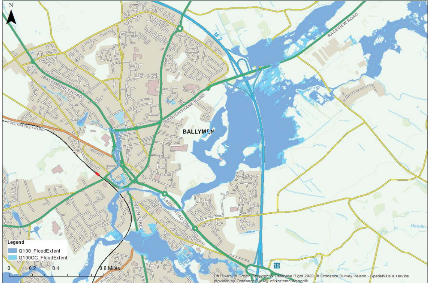
Figure 3-3: Example of Climate Change Flood Hazard Mapping for Ballymena (see turquoise shading)
