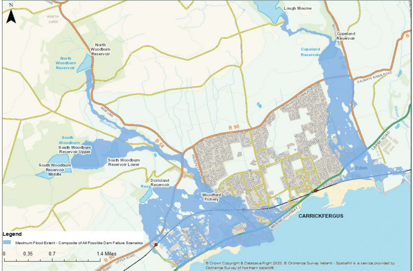
Figure 3-4: Example of Reservoir Inundation Mapping
