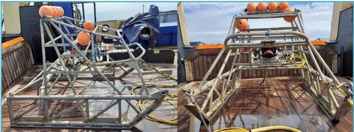
**Figure 3: Photographs showing the AFBI camera sled used during the Summer 2020 surveys.**
