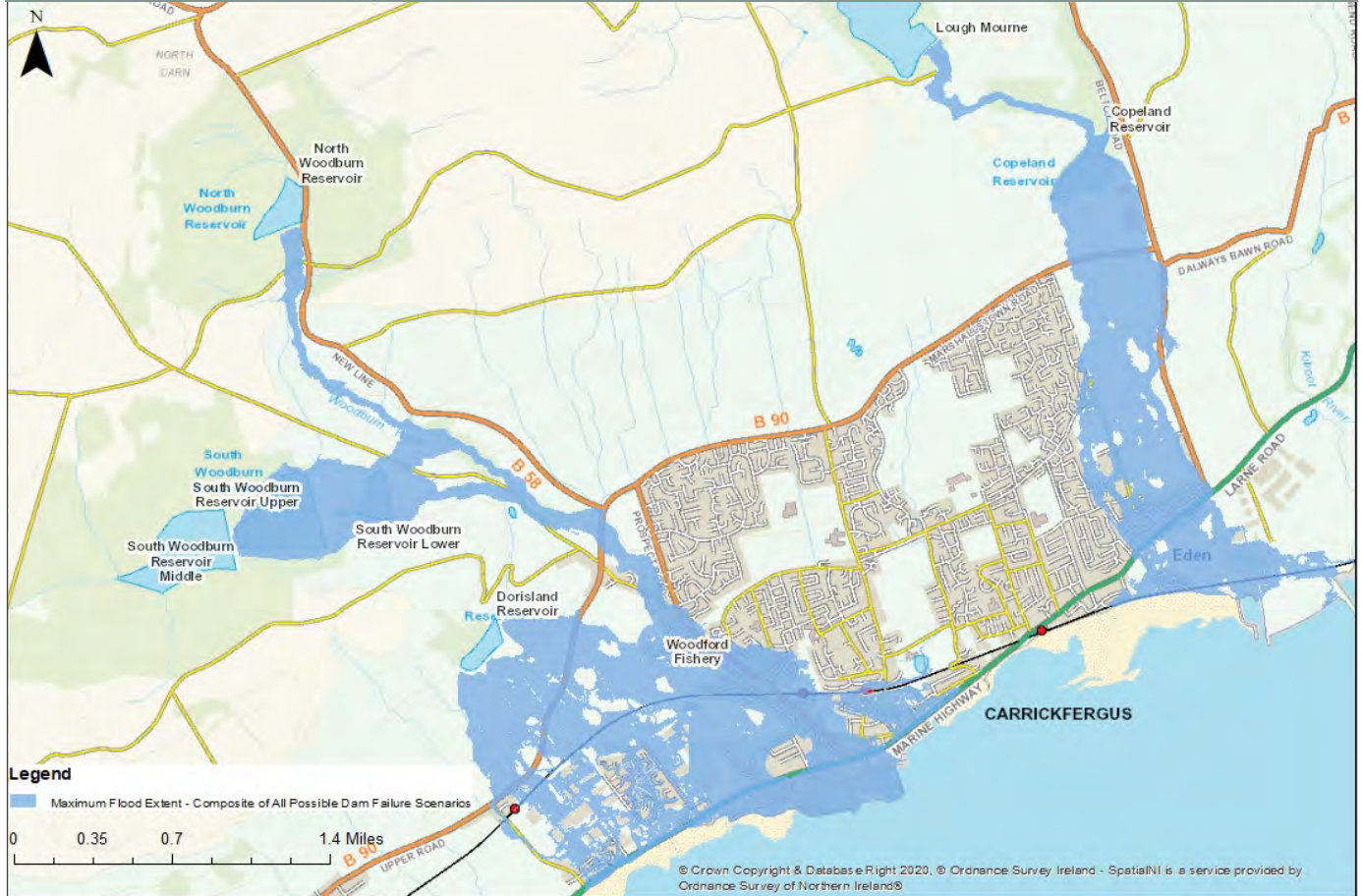
Figure 3-4: Example of Reservoir Inundation Mapping
