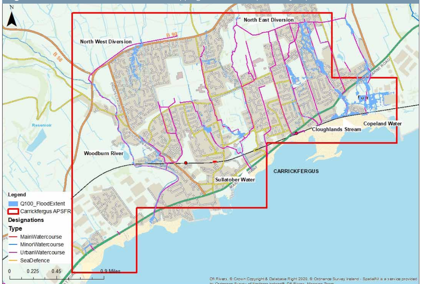
Figure 5.11-8: Overview of fluvial hazard mapping for a 1 % AEP (1 in 100 year) flood event.
