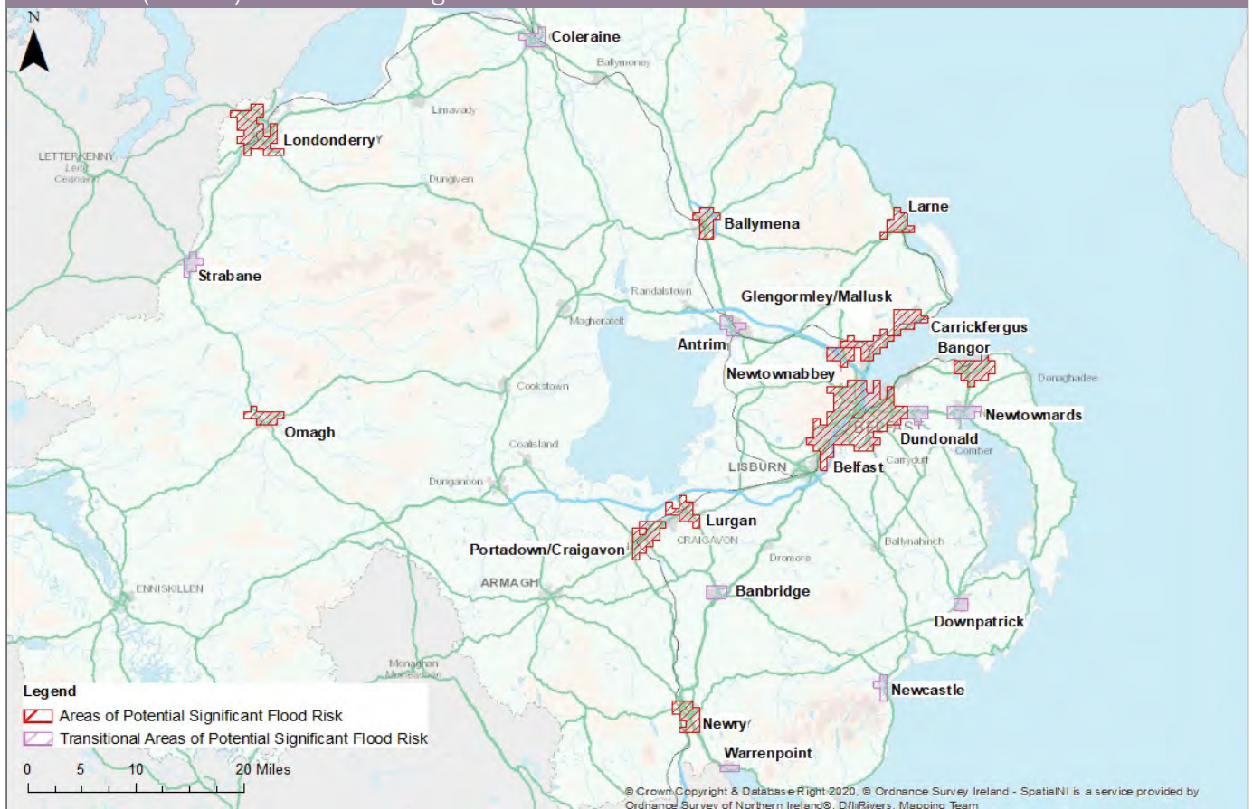
Figure 1-3: Areas of Potential Significant Flood Risk (APSFR) and Transitional Areas of Potential Significant Flood Risk (TAPSFR) as defined through the NIFRA 2018
