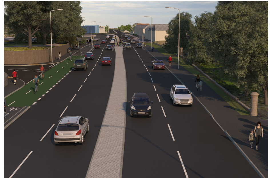
TYPICAL URBAN CROSS-SECTION WITH SEGREGATED CYCLEWAY
