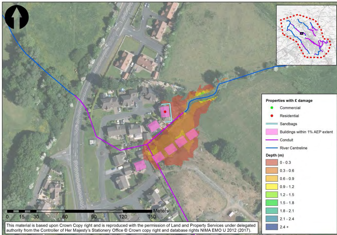
Figure 4.4 - Potential for use of sandbags on Kiln Lodge (Flood Cell 3)
