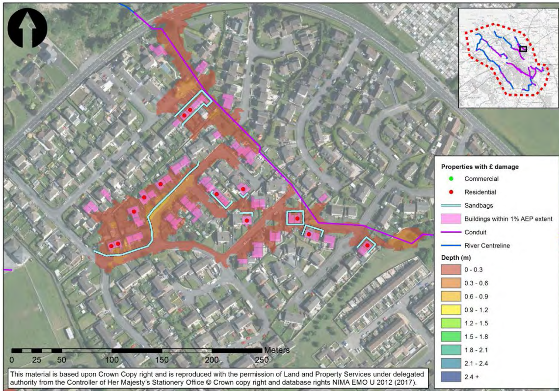
Figure 4.5 - Potential for use of sandbags on residential area off North Circular Road (Flood Cell 4)
