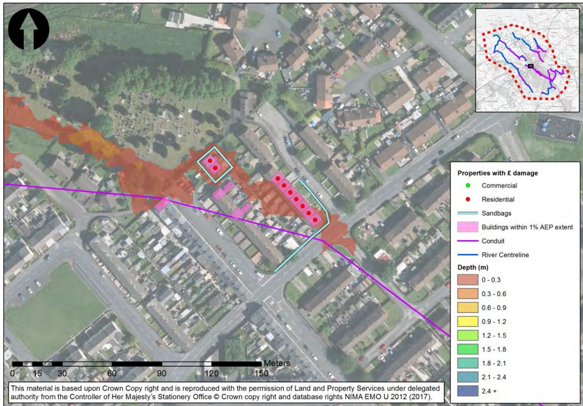
Figure 4.2 – Potential for use of sandbags on Deans Walk and Glebe Terrace (Flood Cell 2)
