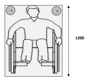
Check that any protrusions into the wheelchair space
