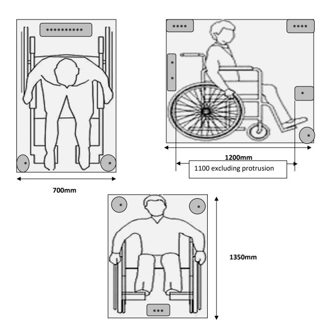
Check that any protrusions into the wheelchair space
