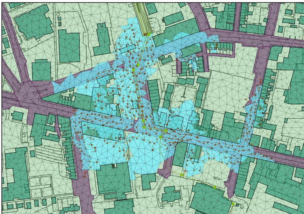
Figure 9.5 Initial Flooding at Upper Edward Street (10hrs 45min model run time)
