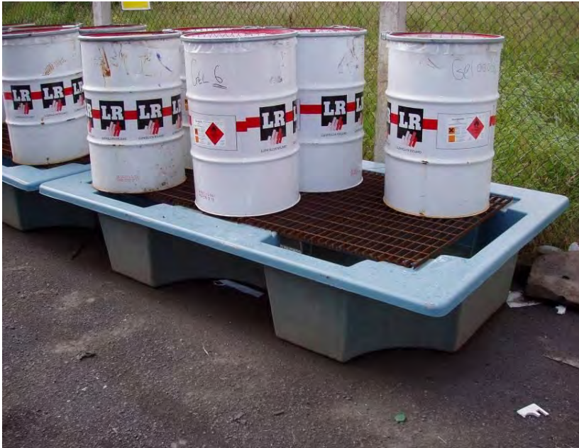
Tank pallet to help capture any leakage
