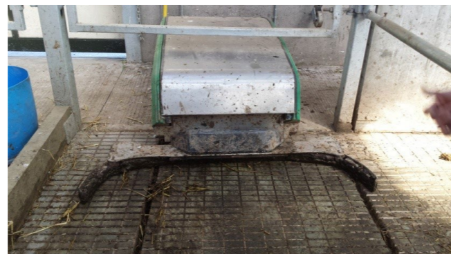
Figure 18: Robotic scraper over grooved floors at CAFRE's Dairy Centre is used to increase scraping frequency and ensure good urine drainage.
