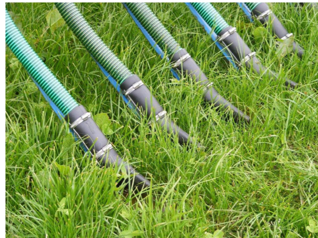
Figure 13a: Close up of the trailing shoe parting the grass and the hose delivering the slurry.
