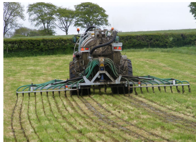
Figure 13b: Trailing shoe slurry application into silage stubble.
