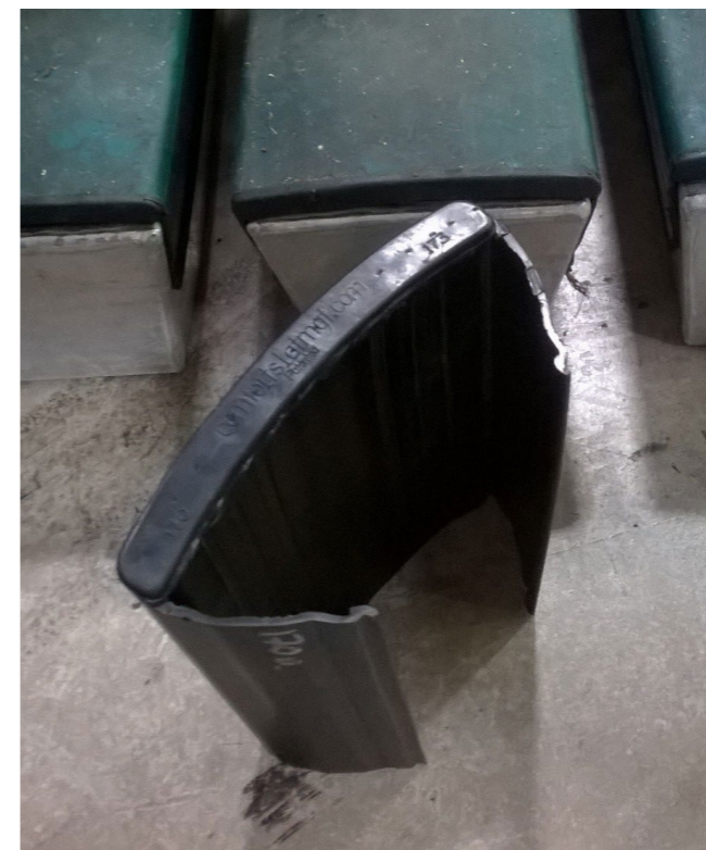
Figure 19: This product can be retrofitted onto existing slats to give a curved upper surface to speed up urine drainage to the tank beneath. It is often fitted over slats to improve animal comfort but it has been found to perform well in reducing ammonia emissions. Flaps can also be fitted which are designed to allow slurry to drop into the tank but reduce fresh air contact with slurry in the tank to minimise ammonia losses.
