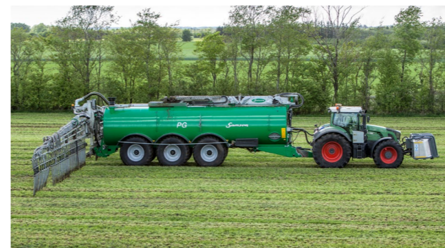
Figure 15: Tanker and tractor with slurry acidification system operated by a contractor in Denmark.
