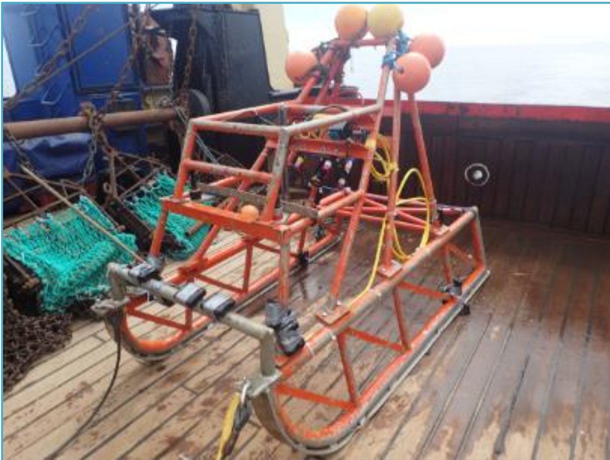
Figure 3: Photograph showing the AFBI camera sledge used during the Summer 2018 surveys.
